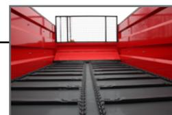
Hydraulic-driven floor (adjustable speed and direction of movement)
