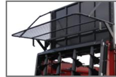
Adapter shield lifted automatically when the back wall (gate) is raised.
